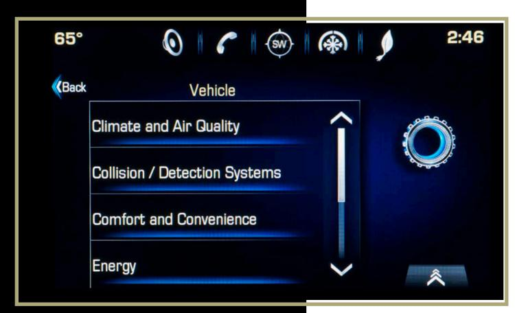
Some vehicle features can be customized using the controls on the infotainment system. The Vehicle Settings menu may include Climate and Air Quality; Collision/Detection Systems; Comfort and Convenience; Energy; Lighting; Power Door Locks; and Remote Lock, Unlock, Start.
